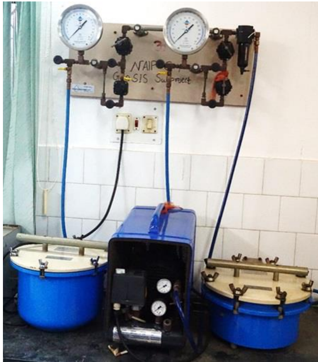
Lab based soil water retention curves (pressure plate method)
