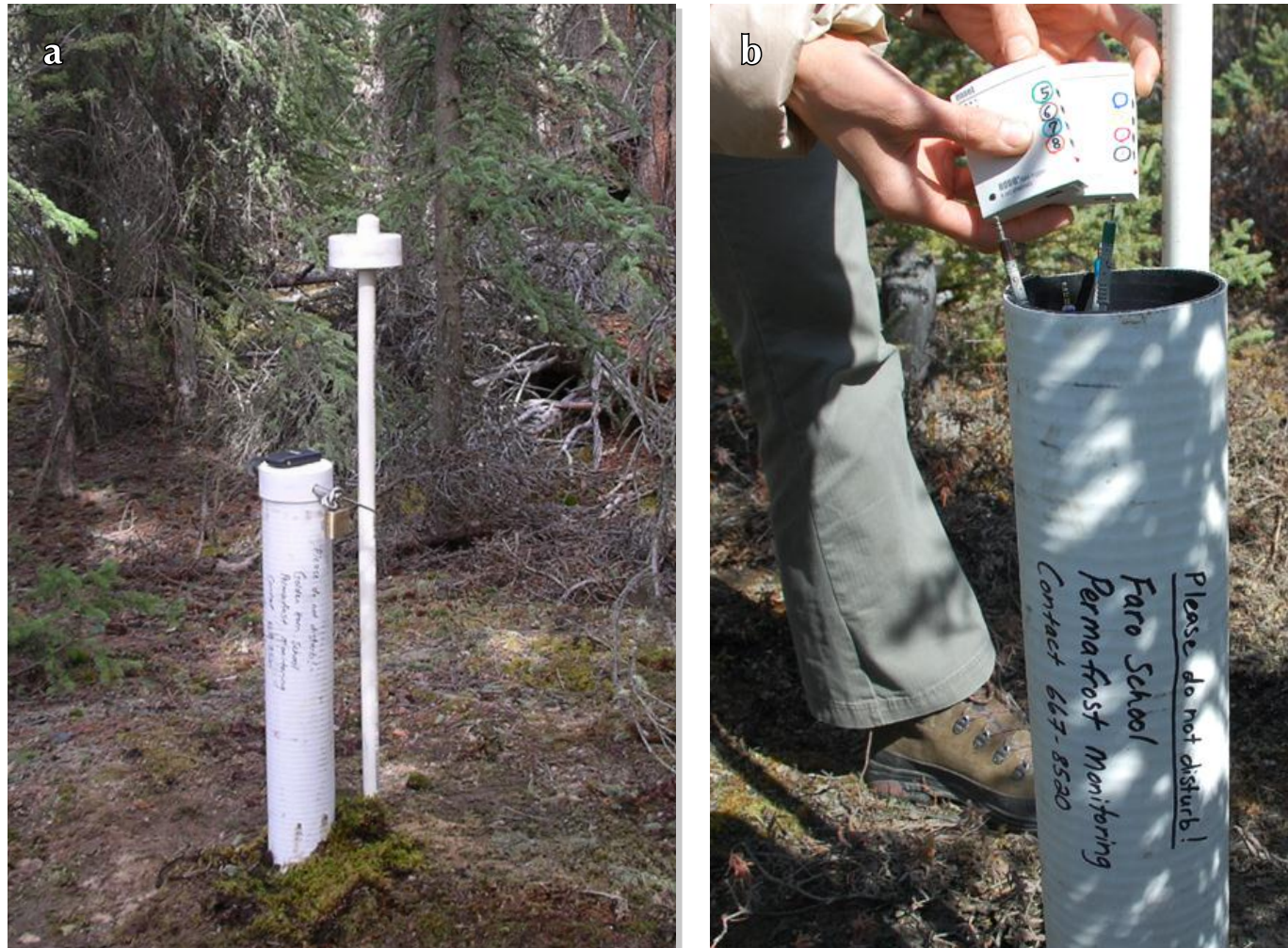
Figure 2. Typical permafrost monitoring station apparatus and configuration. (a) The larger PVC pipe houses the ground temperature sensors and data loggers. The thinner PVC pipe houses an air temperature sensor mounted at 1 m above the ground surface. (b) Four-channel Onset data loggers store hourly temperature measurements for up to 15 months.
