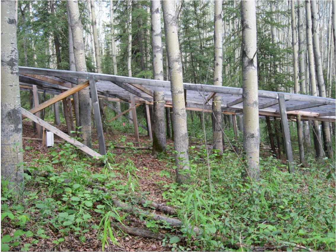
Figure 2.2. Example of the throughfall exclusion treatment. Site depicted in photo is UP2C, an aspen-dominated forest located on 30 degree slope in the uplands. Photo was taken perpendicular to the slope in late August 2007.
